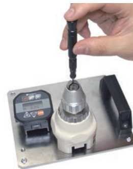
Torque checking figure for AMRD with ATGE-G and measurement stand, #808.
