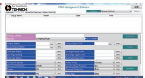
Production tightening mode setting display
