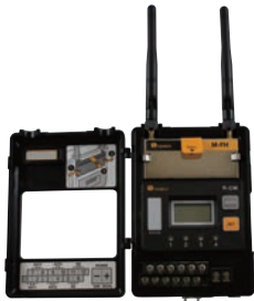
Mounting position of Radio Module
